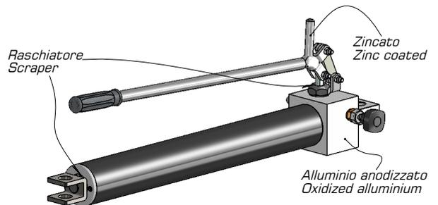
Valvole cementate e rettificatae - Hardened and rectified valves
